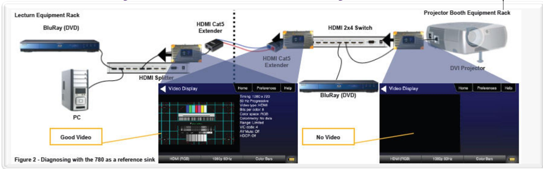
**Test:** Source Test (emulate a known-good HDMI sink) from upstream to downstream
