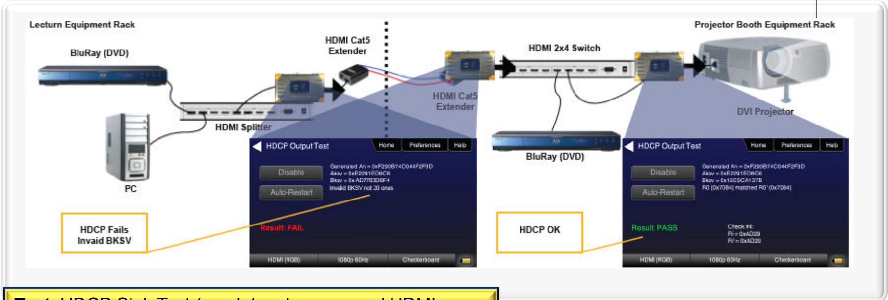
**Test:** HDCP Sink Test (emulate a known-good HDMI source) from upstream to downstream
