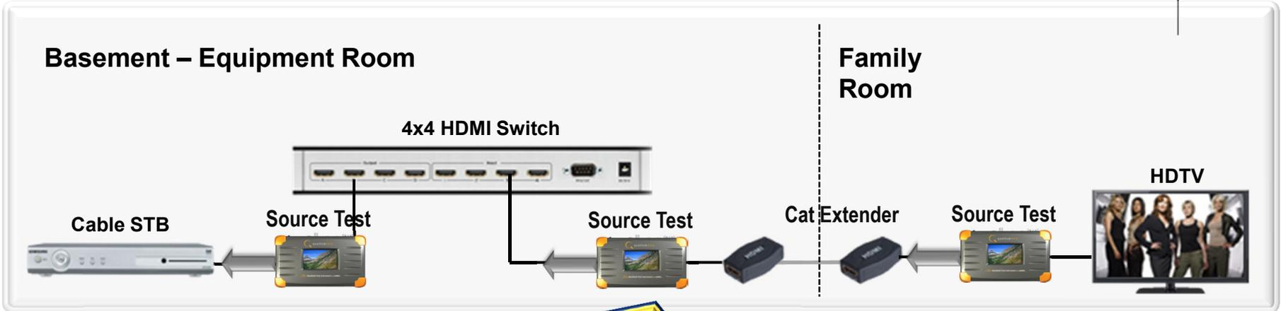
**Test:** Source Test to confirm
