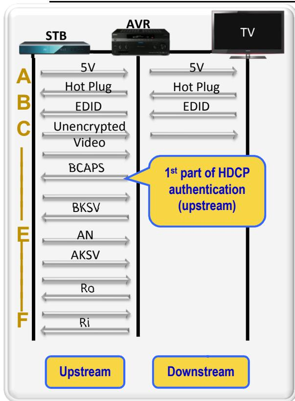
Quantum Data Auxiliary Channel Analyzer - Version 1.40 - DVD1-AVR1-DTV1\_1\_up.BMtrace
