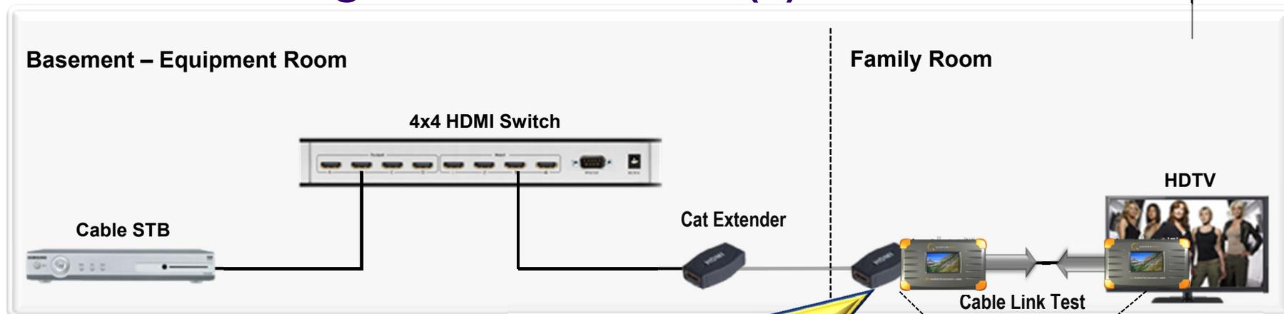
**Test:** Cable/Repeater Test
